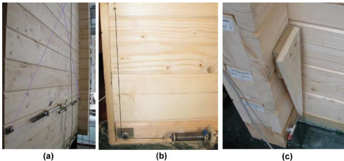
Figure 3.9: LVDT to measure (a) shear deformation (b) wall uplift (c) horizontal sliding
