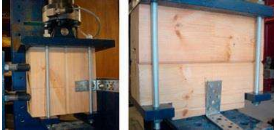
Figure 1.2: Layout of the shear test (left) and tension test (right) performed on connection of the base log and foundation [4]
