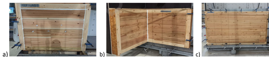
Fig. 3 Test specimens of the watertightness and air permeability tests installed in the testing chamber: NATURLAM W180— a straight specimen and b corner specimen; c TFS 105
